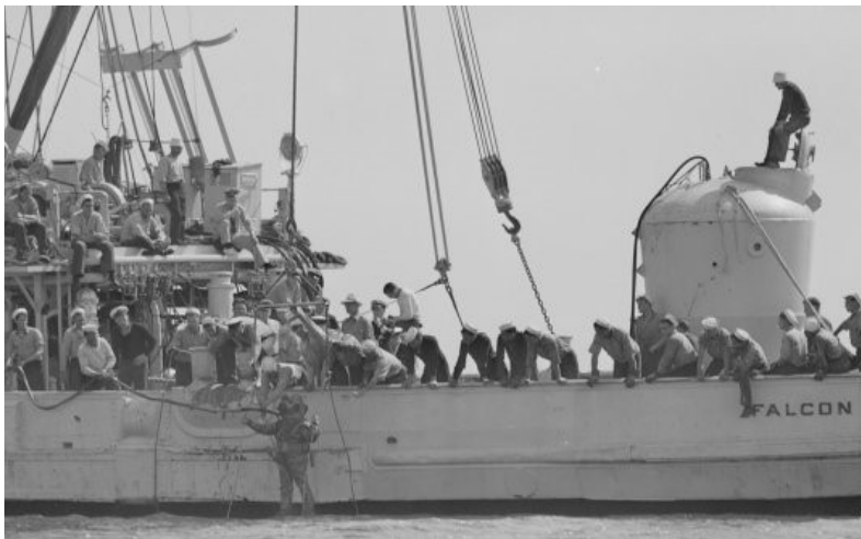
Submarine rescue ship FALCON lowering divers over the side. You can see the Rescue Chamber on the deck, ready to go down.
